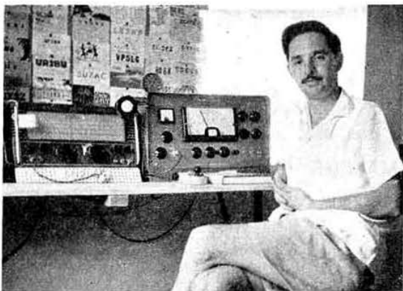
5N2RSB operates this neat station in Kaduna, Nigeria. Equipment includes K.W. Vanguard, Hallicrafters HT17 and B2 transmitters, an Eddystone 750 receiver and an F.B.5 multiband dipole.
